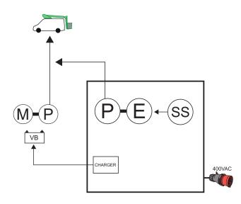
M = Vehicle MotorP = Hydraulic PumpVB = Vehicle BatteriesE = Electric Motor
